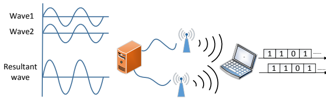
Figure 1: Constructive interference of two waves.
